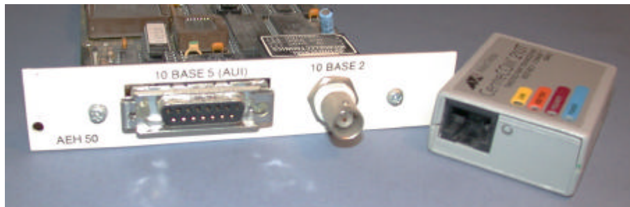
fig 8 NIC with 10 base 5 and 10 base 2 connectors, with AUI for 10 base T
