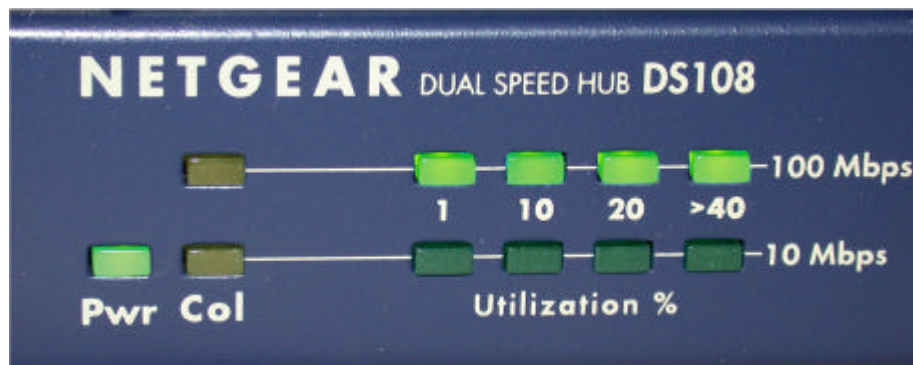
fig 10 High network bitrate, with no collisions
