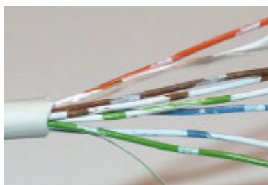
fig 6 Wire colours for standard RJ45 cable
