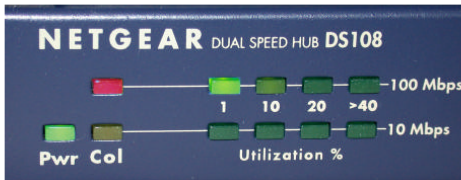
fig 9 Ethernet packet collision occurring at low utilisation
